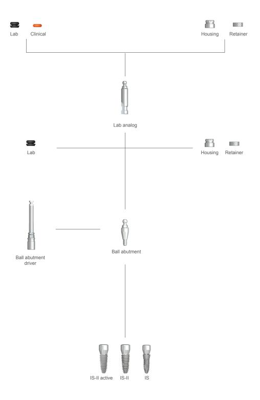
Note. When abutments are connected to Narrow Fixture(Ø3.5) or Short Fixture(7.3mm), the total height of abutment is 0.4mm higher than Regular-Wide cases.
